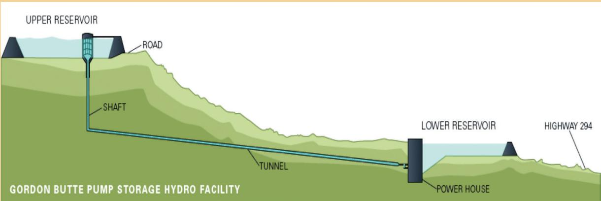
An artist's rendering at top shows the two reservoirs in relation to each other. The pools of water are connected by a penstock, and turbines power a generator. Gravity pulls water down to the lower reservoir when the electrical grid needs energy. At times of low usage, water can be stored above, where the reservoir essentially acts as a battery. Unlike wind and solar energy, which have gaps, the hydro loop can be responsive to demand, whatever the weather.
